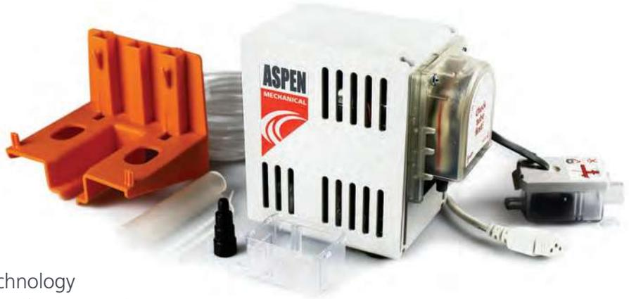
Bringing mini pump and peristaltic pump technology together. Simply position the remote reservoir (float switch) in the condensate tray or fix to the drain-pipe connection (depending on chosen reservoir). Alarm option available.
