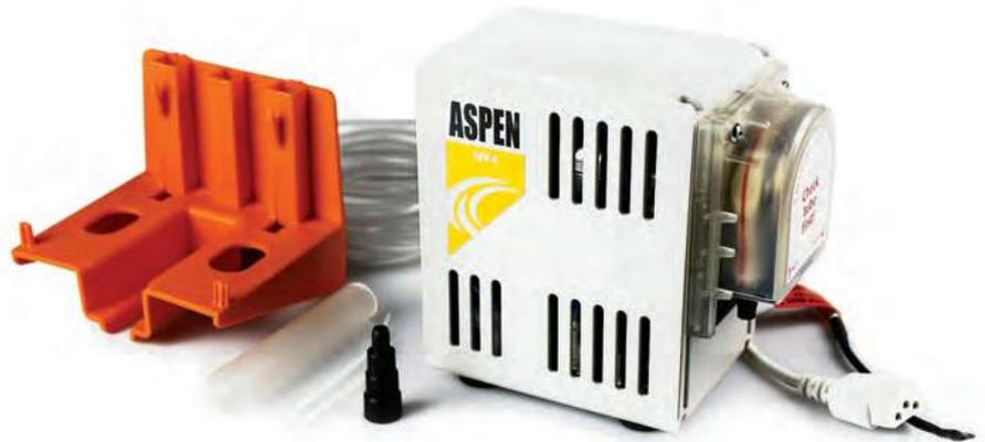
The MK4 peristaltic is operated using two water sensors. The lower sensor comes into contact with water, the heat conductivity from that sensor provides a temperature difference between the second – energising the pump.
