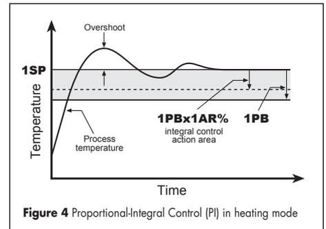
**4.3.3. PROPORTIONAL-INTEGRAL-DERIVATIVE CONTROL.** Response overshoot in a system controlled by a PI controller may be reduced by inserting a derivative action in the control. The derivative action is greater the faster the temperature variation within the time unit. A controller with a high derivative action (**1DT** high) is extremely sensitive to small temperature variations and can make the system unstable. With **1DT=0** the derivative control is disabled.
